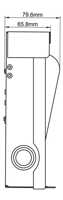
The dimention of the switch in the product of the PDS-30A,PDS-60A,PDS-60AN is the same, but the fuse is different . as follow:
